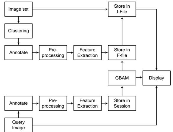
Figure 1. Schematic block diagram of the CBIR system
