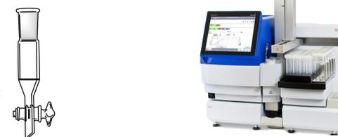
Figure 3. Traditional SPPS vessel and Biotage® Initiator+ Alstra™ peptide synthesizer.
