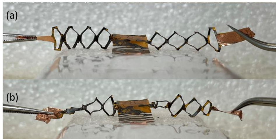
Fig. 12: Kirigami Sensor tested under (a) 180° twisting; (b) 360° twisting
