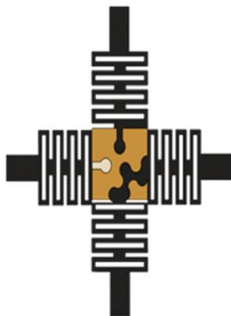
Fig. 8. Kirigami shaped Sweat pH and Skin Temperature Sensors
