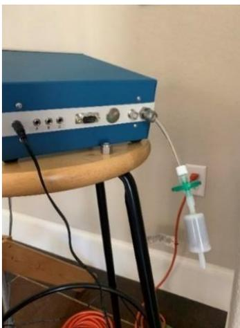
*Figure 40. Ozone scrubber attached to ozone monitor*
