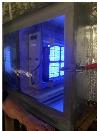
*Figure 31. PCO A core (left) and in plenum (right)*
