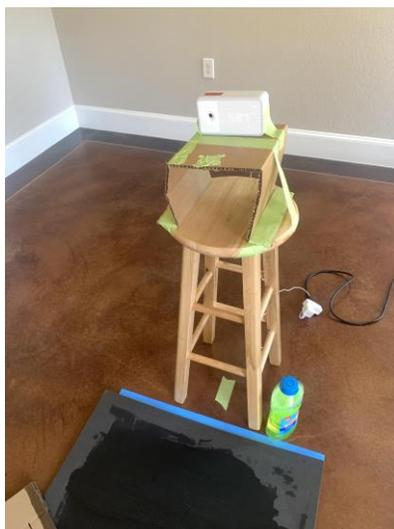
*Figure 28. Setup for Mr. Clean all-purpose cleaner VOC injection*
