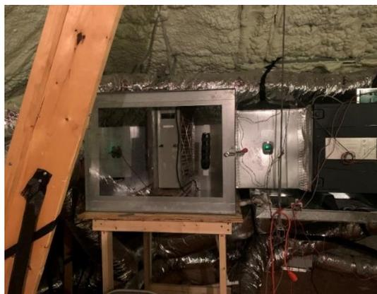
*Figure 24. Plenum setup used to evaluate PCO air cleaners*
