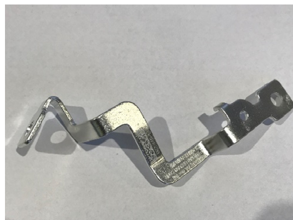
Figure 3. Aluminum (EN AW 5005A-H24) Busbar ground connection galvanized by (Cu: 3 +3/0) \mu\text{m} . (Sn: 7 +4/0) \mu\text{m} .
