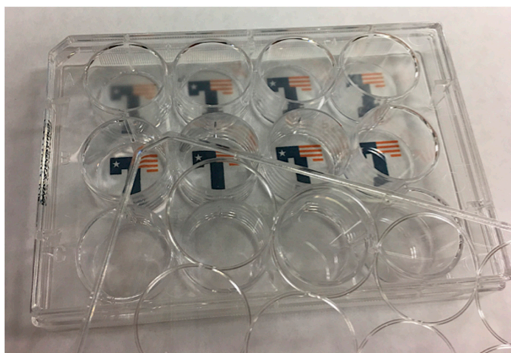
Figure 1. Physical appearance of the four polyurethane (PU) films: From left to right in the top wells, 200ET, 100ES, 60ES, and 60ET. The second row of four wells contains no PU films for comparison of the transparency of the PU films.
