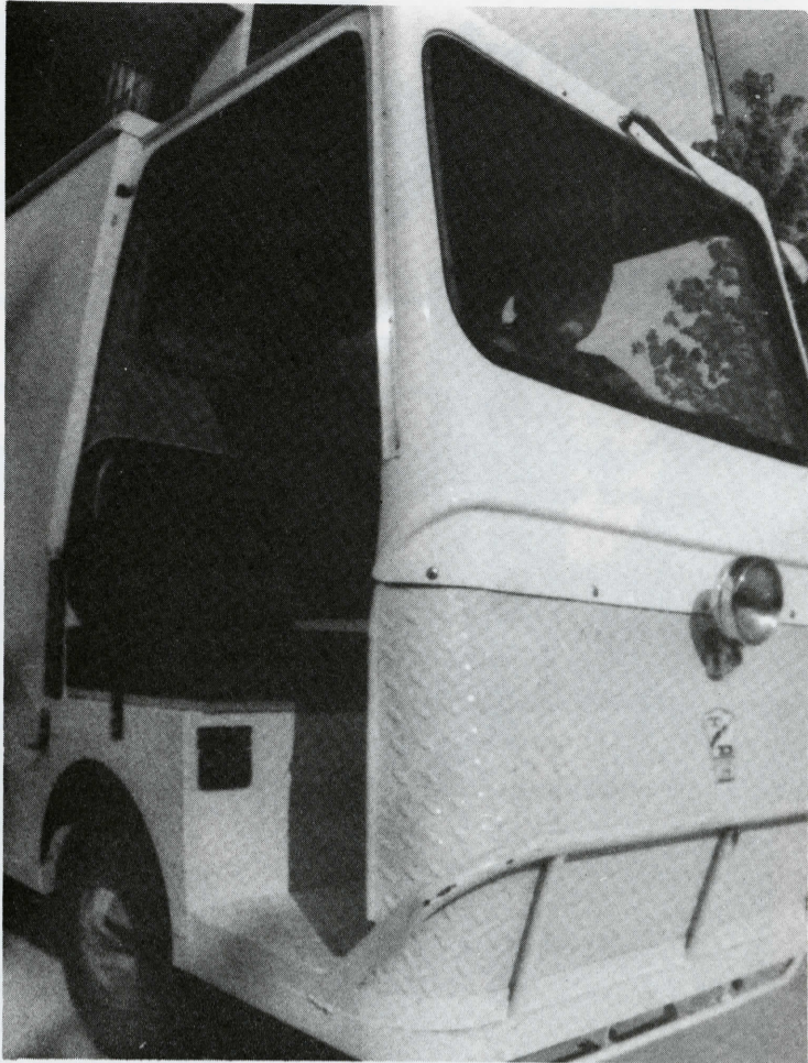
SPEEDY SERVICE — Ben Ferrell Jr., media center audio visual technician III, shows off the new Taylor-Dunn enclosed burden carrier. The electrical vehicle, which will carry up to 2,000 pounds and two passengers, is part of the equipment for the new library.
