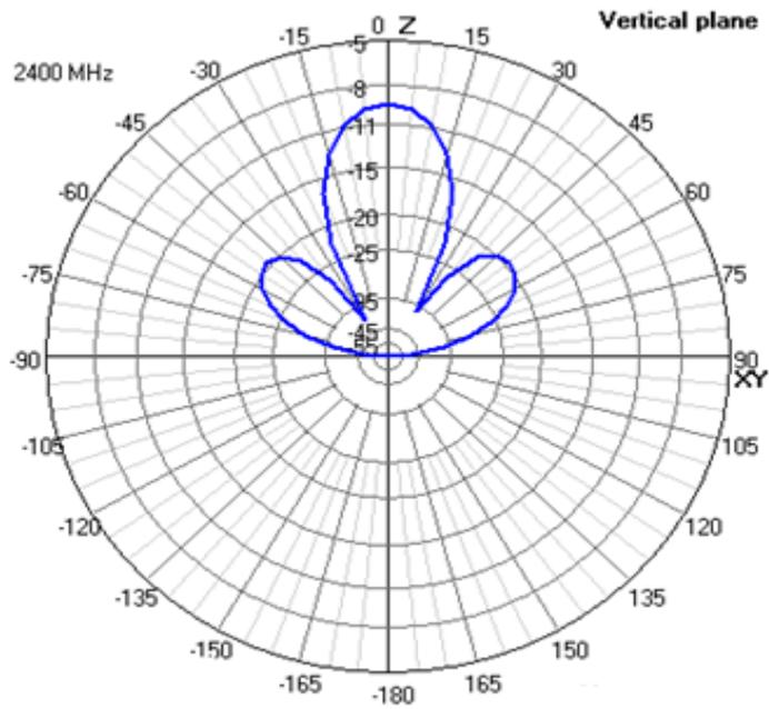
Figure 20. Radiation pattern showing the vertical gain in the vertical plane.
