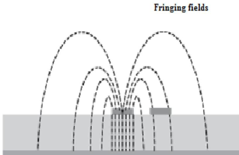
Figure 6. Fringing fields of a microstrip antenna.
