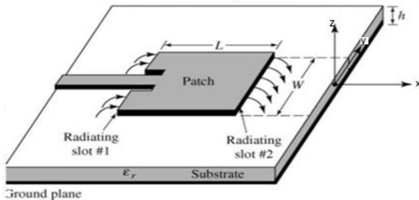
Figure 1. The geometry of a Microstrip antenna patch [3]
