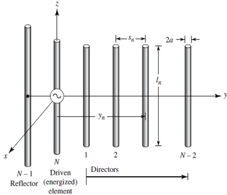
Figure 15. Yagi-Uda antenna with directors and reflector elements [3].
