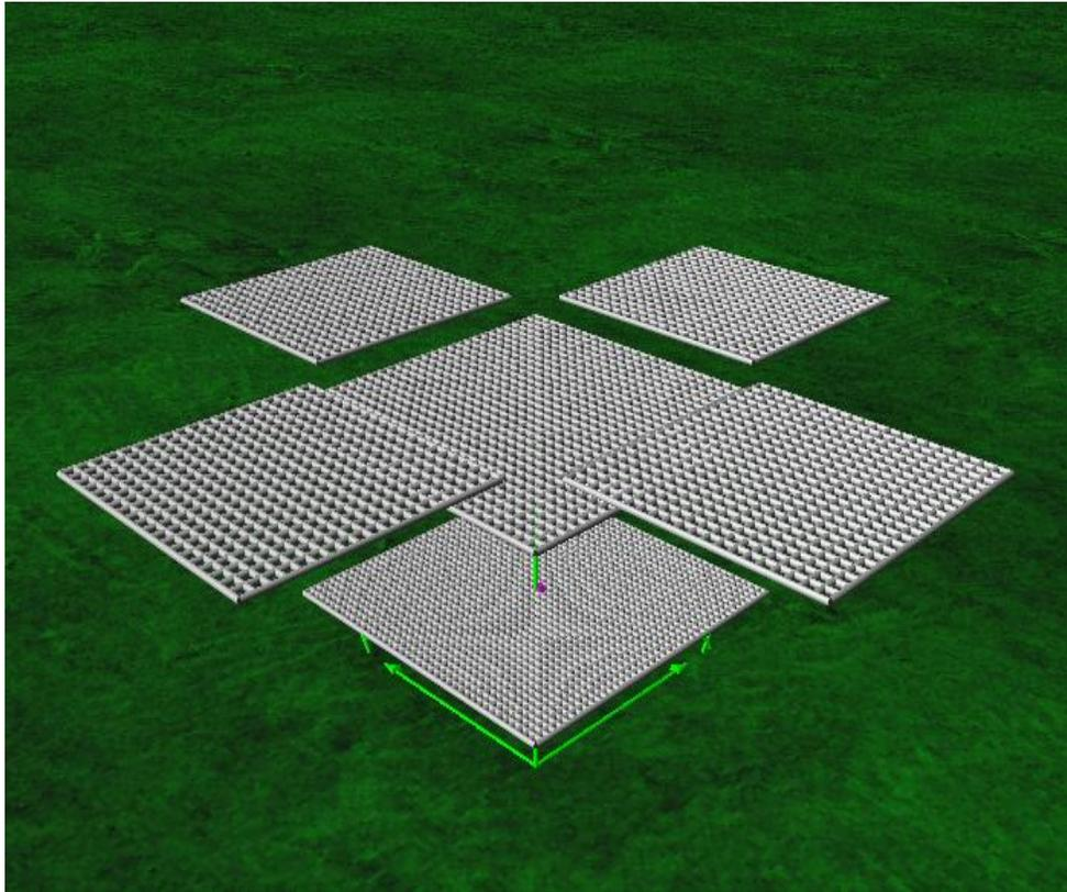
Figure 16. 3-D view of the antenna design
