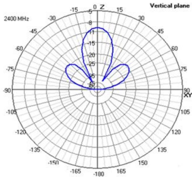
Figure 27. Radiation pattern showing total gain in the vertical plane
