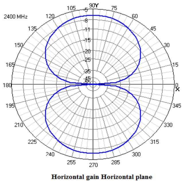
Figure14. Radiation pattern showing horizontal gain in the horizontal plane.
