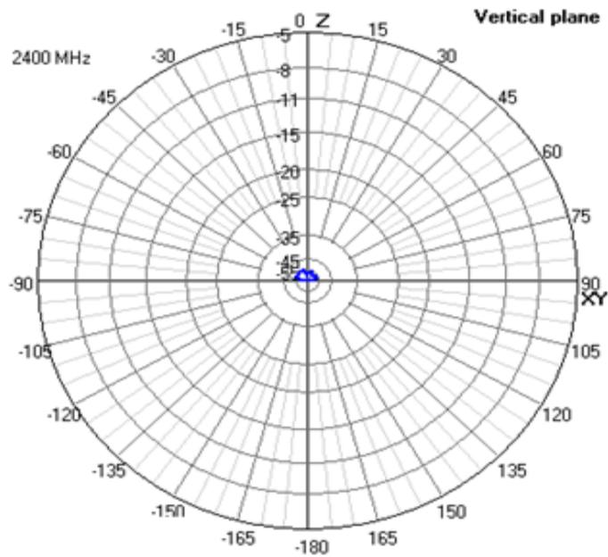
Figure 24. Radiation pattern showing horizontal gain in the vertical plane
