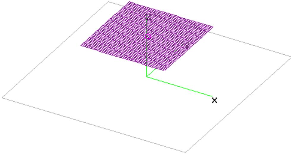
Figure 8. 3- D view of the designed microstrip antenna.
