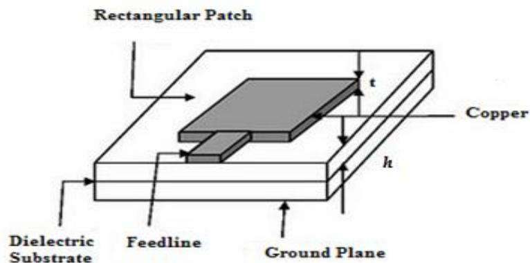
Figure 3. Rectangular patch microstrip antenna
