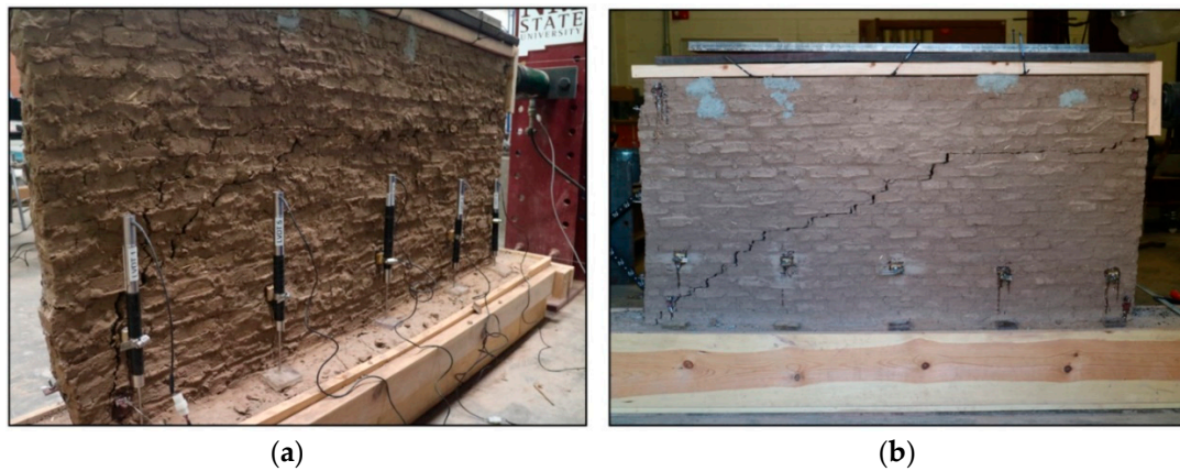
Figure 6. Wall 1: (a) During loading; (b) after failure (after test completion).
