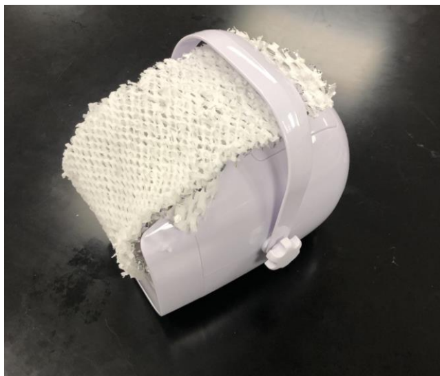
Figure 3. Modified bubble machine for generation of hydrogen peroxide vapor.
