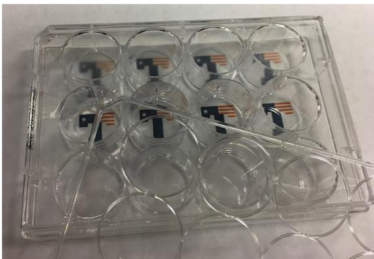
Figure 4. Physical appearance of the four commercial PU films: from left to right in the top wells, 200ET, 100ES, 60ES, and 60ET. The second row of 4 wells contains no PU films for comparison of the transparency of the PU films.
