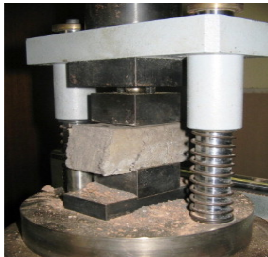
Figure 2.1: Adobe Specimen Tested in Compression
