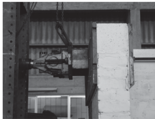
Figure 2.4. Application of load in the wall (Blondet, 1978)
