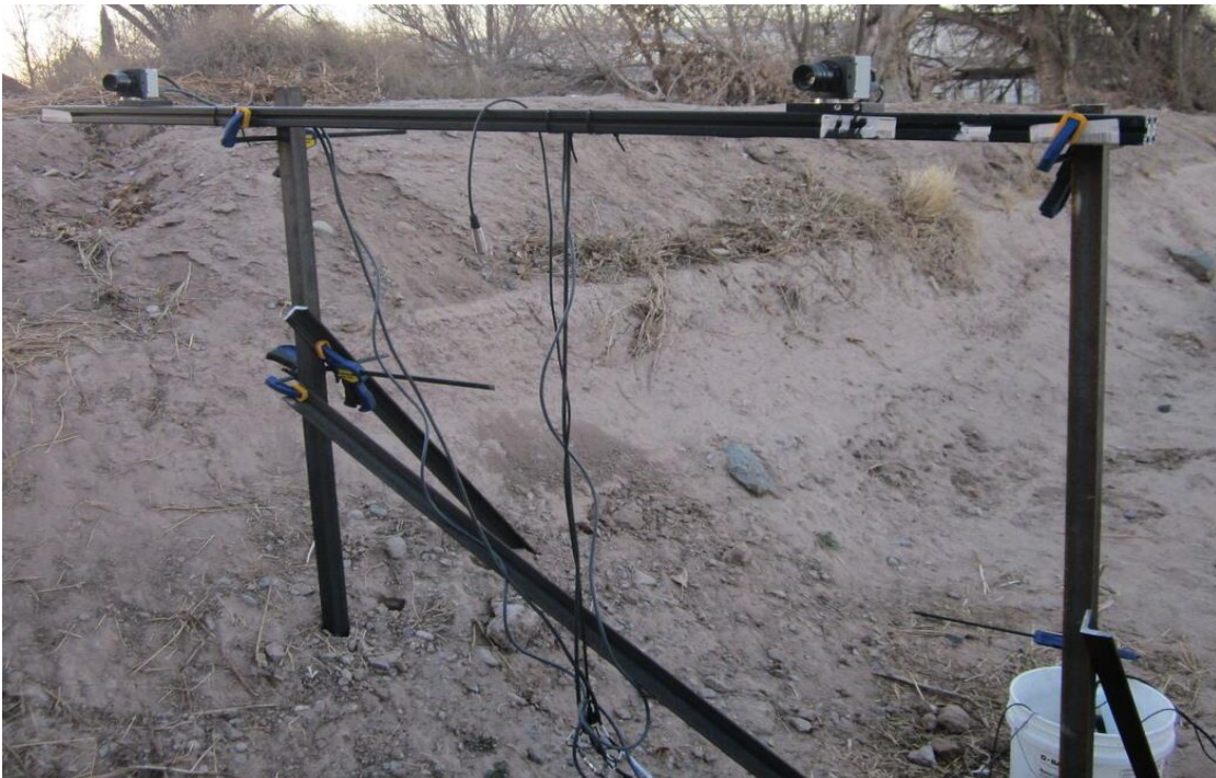
Figure 7. FASTEC HiSpec1 System for monitoring exterior girder of HPC span
