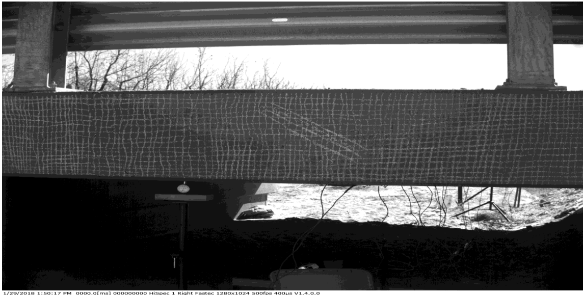
Figure 27. Pattern drawn on UHPC beam (fascia girder) picture taken from right camera
