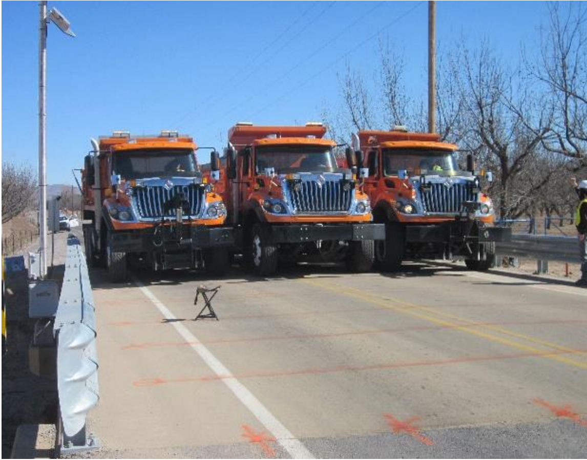
Figure 5. Example of truck positioning with (a) one truck, (b) four trucks back-to-back, (c) three trucks side by side
