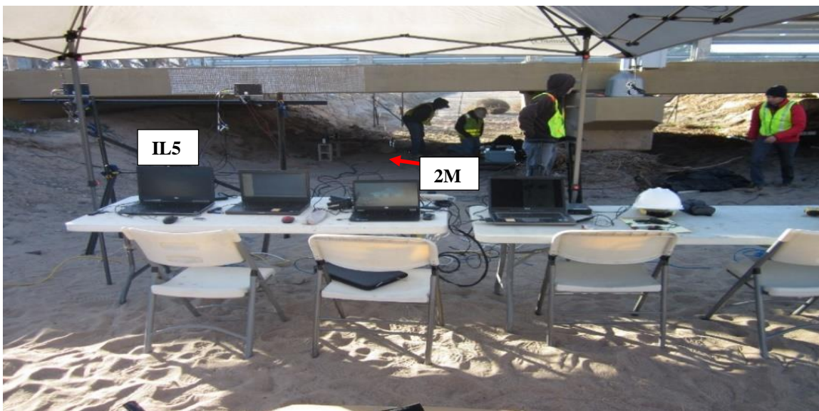
Figure 13. Command station with computer systems running DIC cameras
