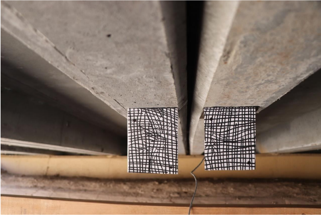
Figure 28. Pattern with high contrast attached to the internal girder
