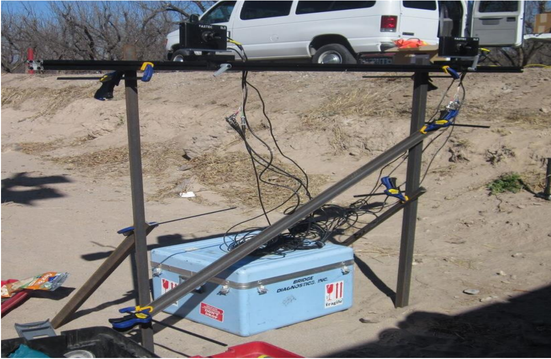
Figure 6. FASTEC IL5 System for monitoring exterior girder of UHPC span
