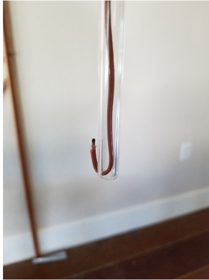
Figure B1. Thermocouple hanging through acrylic tubing
