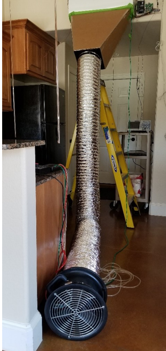
Figure B9. Airflow validation setup
