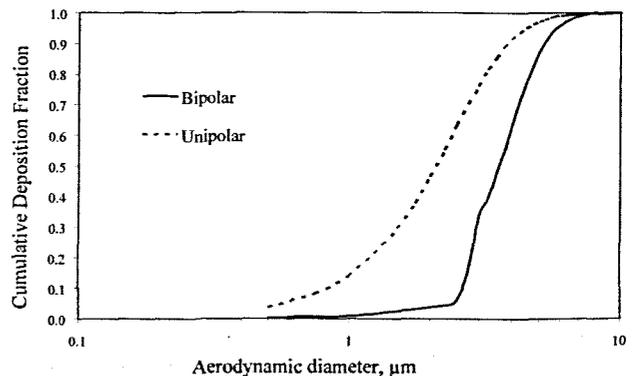
Fig. 6. Comparison of the respiratory deposition fraction of bipolar charged versus unipolar charged aerosols in the glass bead tracheobronchial model airways.
