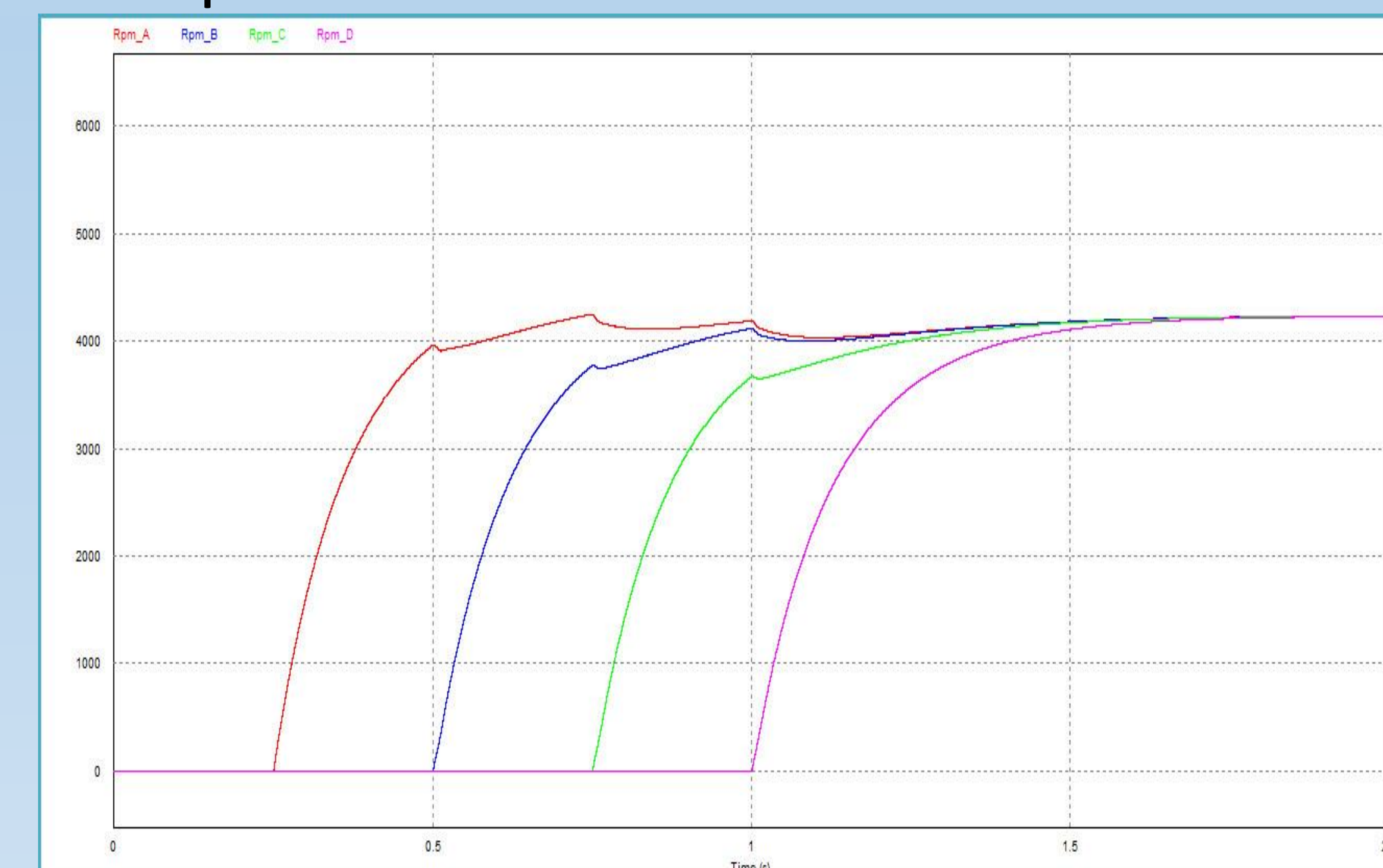
Speed output of 4 motors using PI Control only
